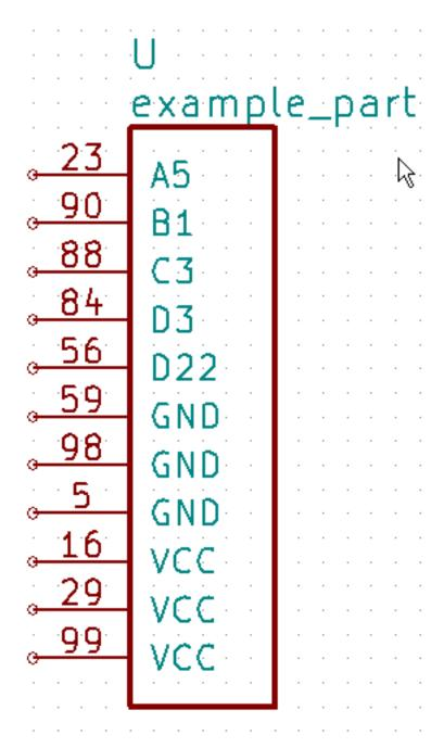
The command kipart  $\neg$ b example.csv  $\neg$ o example4.lib will bundle power and no-connect pins with identical names (like GND, VCC, and NC) into single pins like so:
