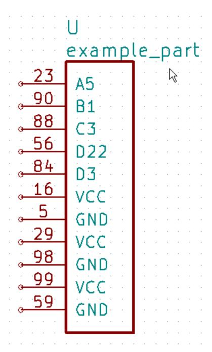
The command kipart -s num example.csv -o example2.lib will create a schematic symbol where the pins are arranged by their pin numbers:
