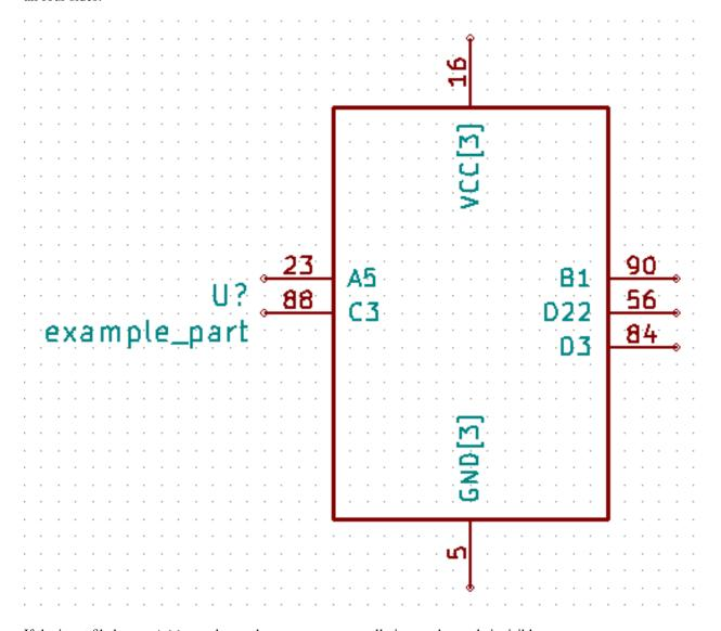
If the input file has a Hidden column, then some, none, or all pins can be made invisible:
