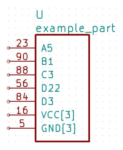
Or you could divide the part into two units: one for I/O pins and the other for power pins by adding a Unit column like this:
