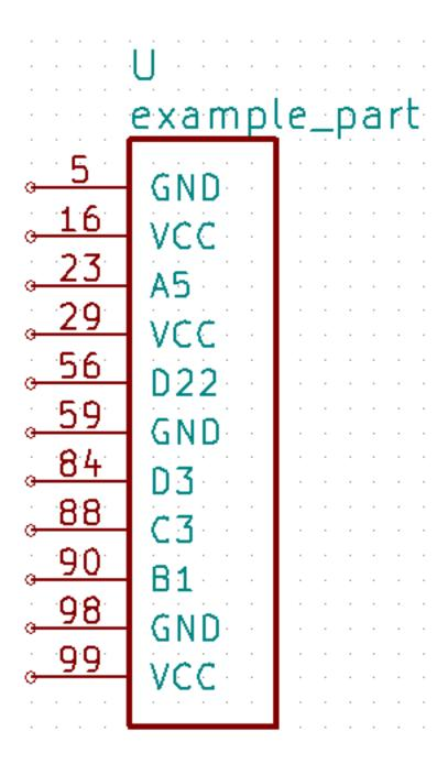
The command kipart -s name example.csv -o example3.lib will create a schematic symbol where the pins are arranged by their names:
